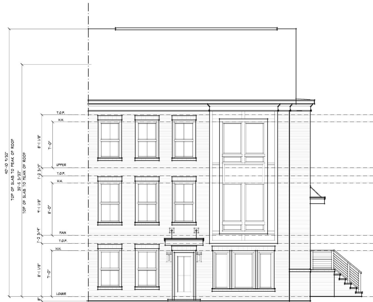
UNIT C: FRONT ELEVATION #1 1/4"=1'-0"
