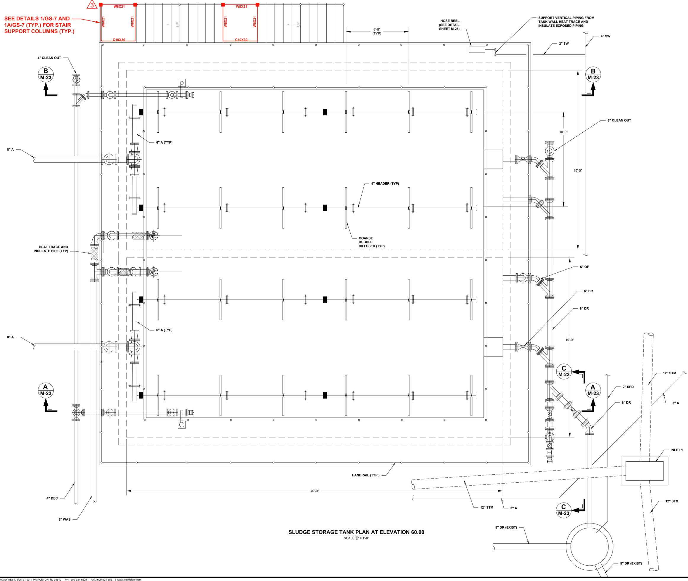
SLUDGE STORAGE TANK PLAN AT ELEVATION 60.00
