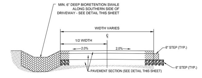
**PROPOSED ACCESS DRIVEWAY PAVEMENT CROSS-SECTION (TYP)**
