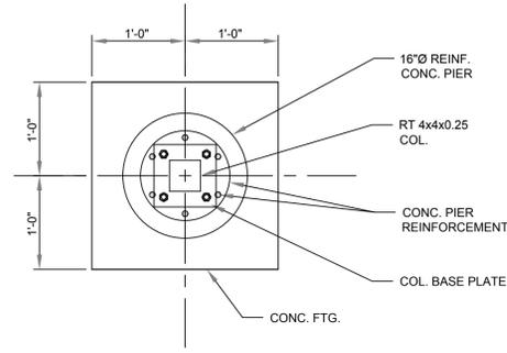
1A TYPICAL NEW PLATFORM FOOTING - PLAN
