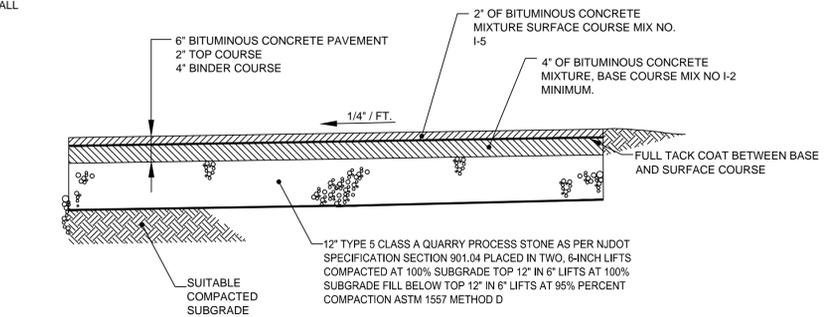
**PROPOSED ACCESS DRIVEWAY PAVEMENT SECTION (TYP)**
