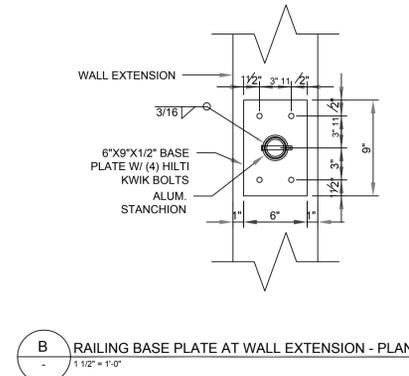
B RAILING BASE PLATE AT WALL EXTENSION - PLAN
