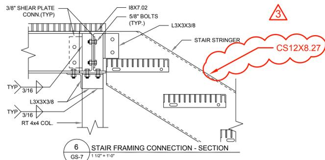
6 STAIR FRAMING CONNECTION - SECTION
