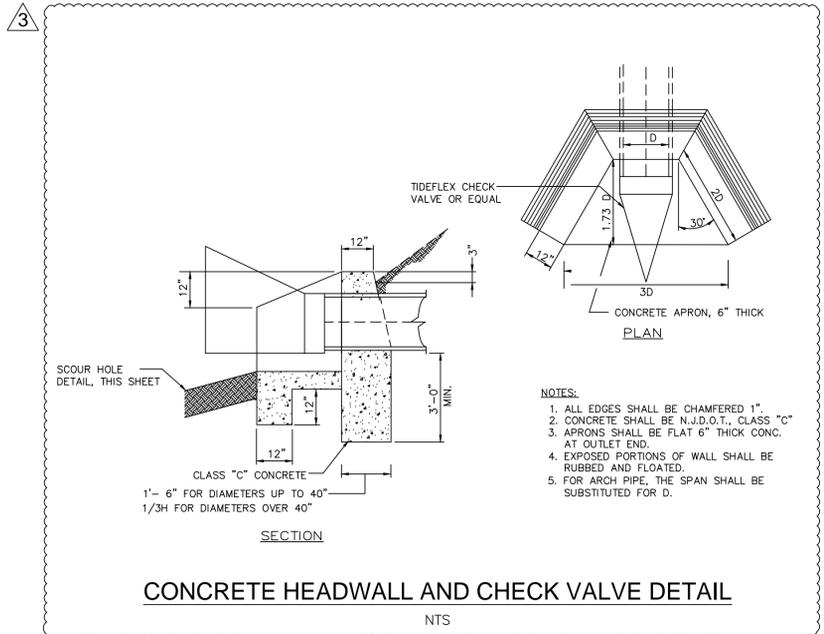
**CONCRETE HEADWALL AND CHECK VALVE DETAIL**
