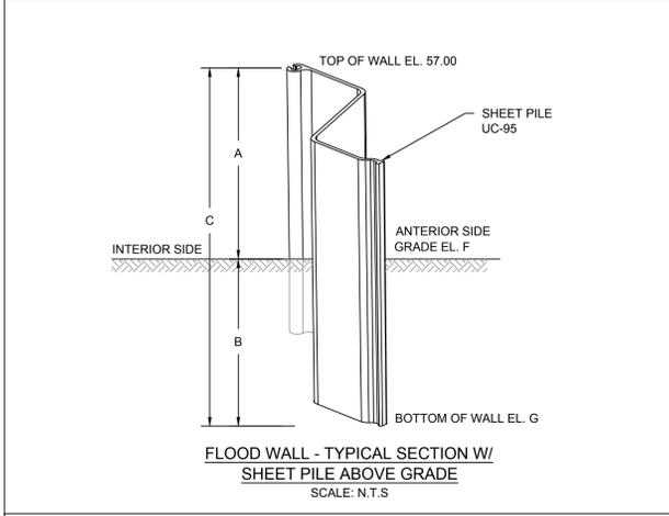
FLOOD WALL - TYPICAL SECTION W/
