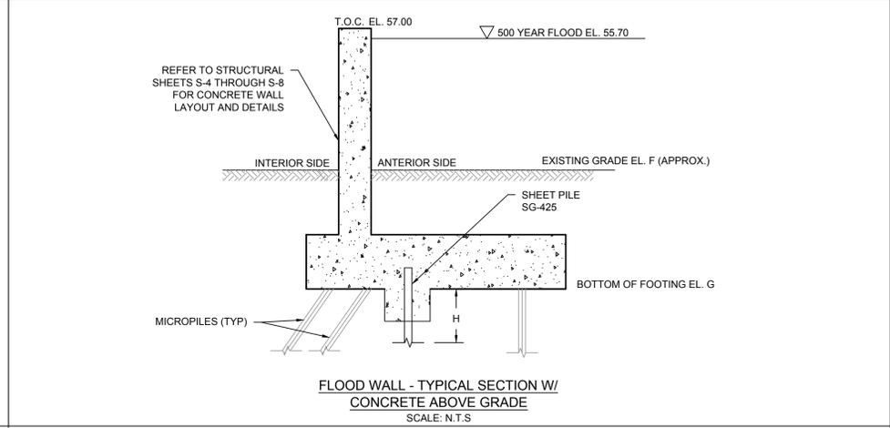
FLOOD WALL - TYPICAL SECTION W/
