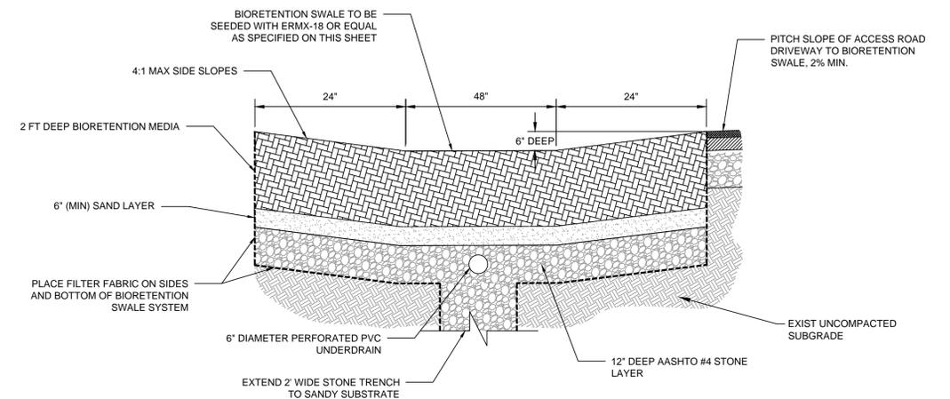
**BIORETENTION SWALE DETAIL**
