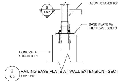
2 RAILING BASE PLATE AT WALL EXTENSION - SECTION
